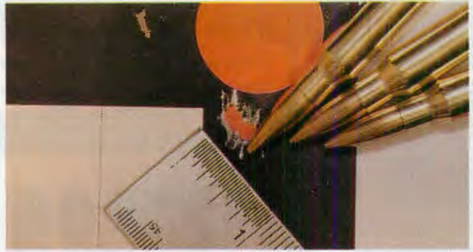
Teamed with good ammunition our Steyr proved capable of superb accuracy as this .20-inch, 100-yard, three-shot group attests.
